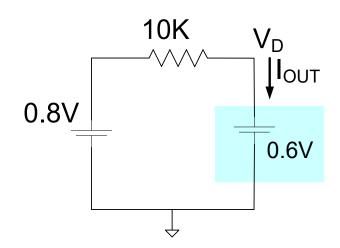
Solve simultaneously, assume V<sub>t</sub>=25mV, I<sub>S</sub>=1fA
