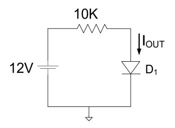
$$I_{\text{OUT}} = I_{\text{S}} \left( e^{\frac{-I_{\text{OUT}} \bullet 10K}{V_{\text{t}}}} e^{\frac{12}{V_{\text{t}}}} - 1 \right)$$
