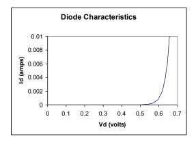
I<sub>S</sub> in 10fA -100fA range (for signal diodes)
