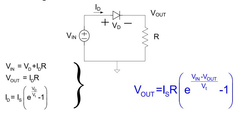
This analysis is rigorous (using only KVL and device models)
