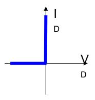
Analysis based upon "passing current" in one direction and "blocking current" in the other direction
