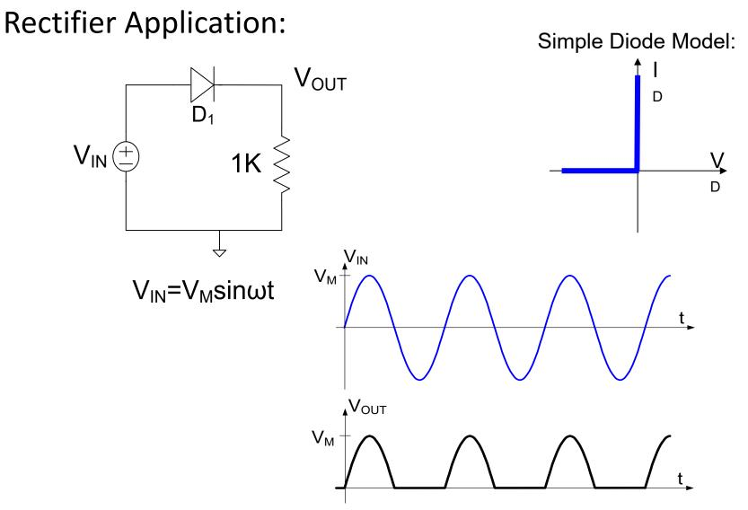
Analysis based upon "passing current" in one direction and "blocking current" in the other direction
