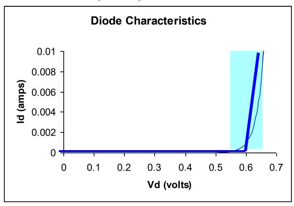
Better model in "ON" state though often not needed Includes Diode "ON" resistance
